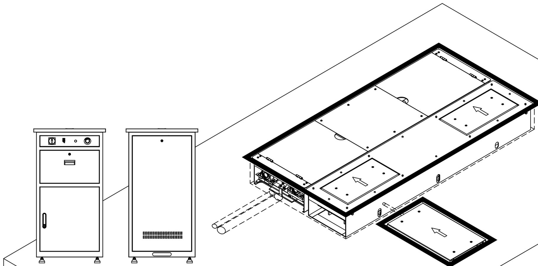
Tidy up the motor power cable and signal cable inside the bench, use cable tie if needed, cover and tighten all bench cover plates;
