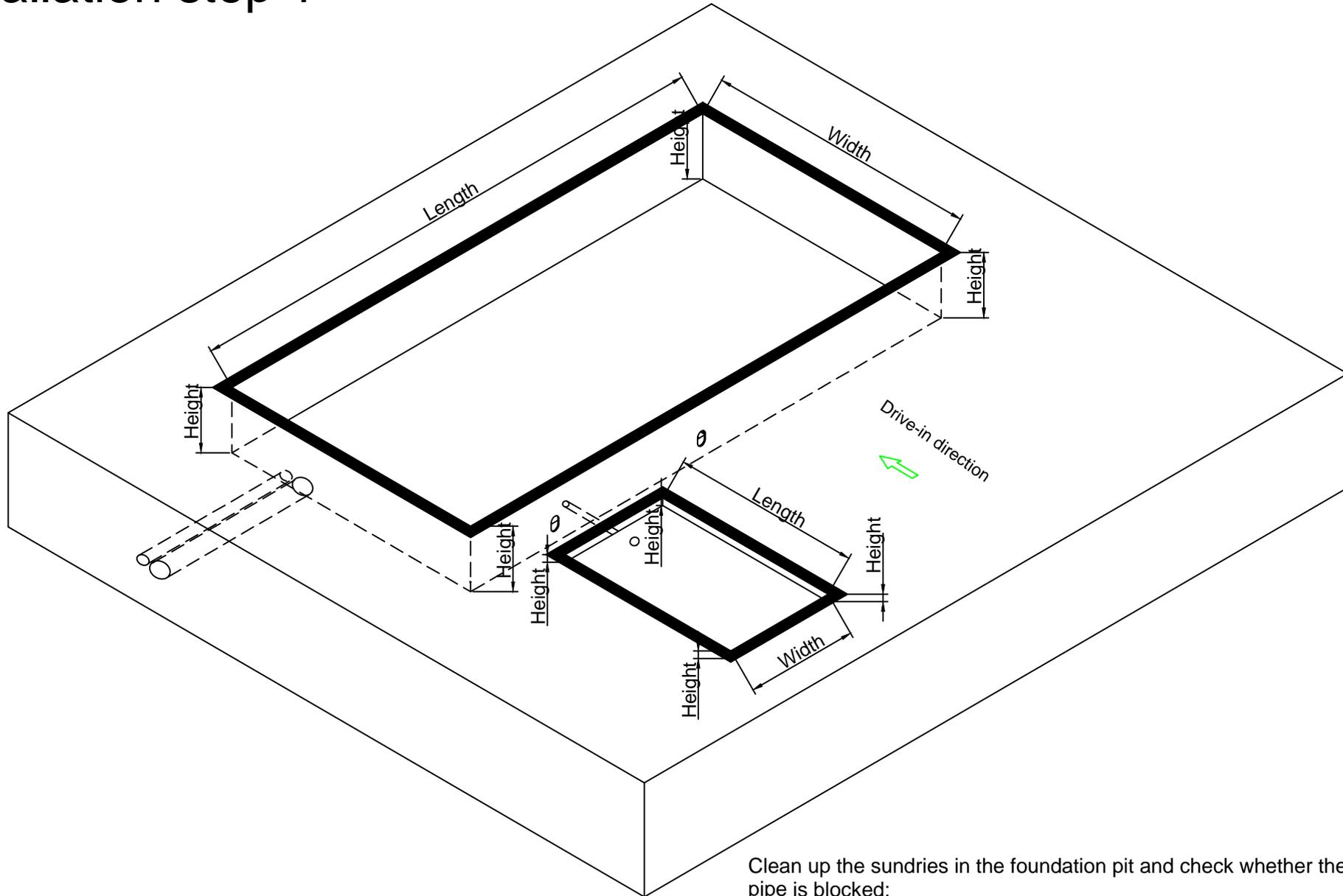
Clean up the sundries in the foundation pit and check whether the embedded pipe is blocked;
