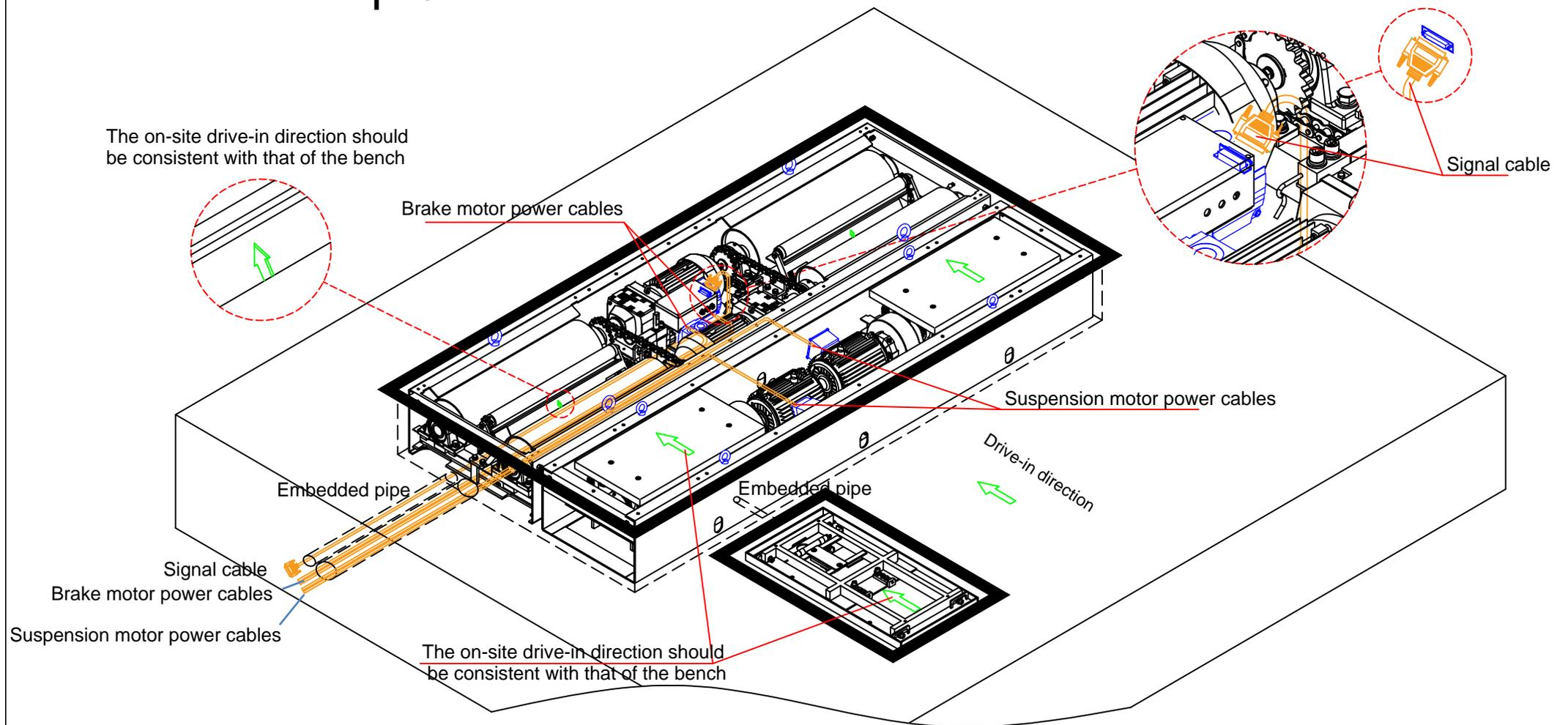
Hoist the bench into the foundation pit, and make sure the on-site drive-in direction is consistent with that of the bench;
