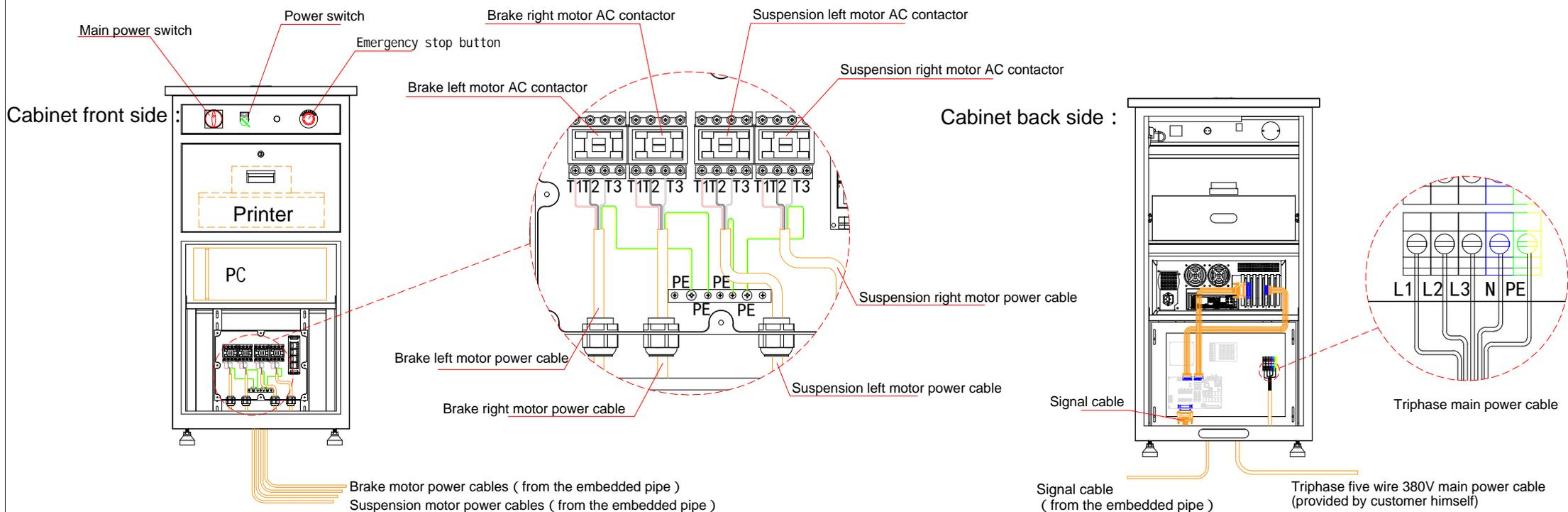
Before start the wiring, make sure that the main power switch and the power switch are turned to "off", and press the emergency stop button. Remove the panels of both front and back side, open the panel of the back junction box ;
