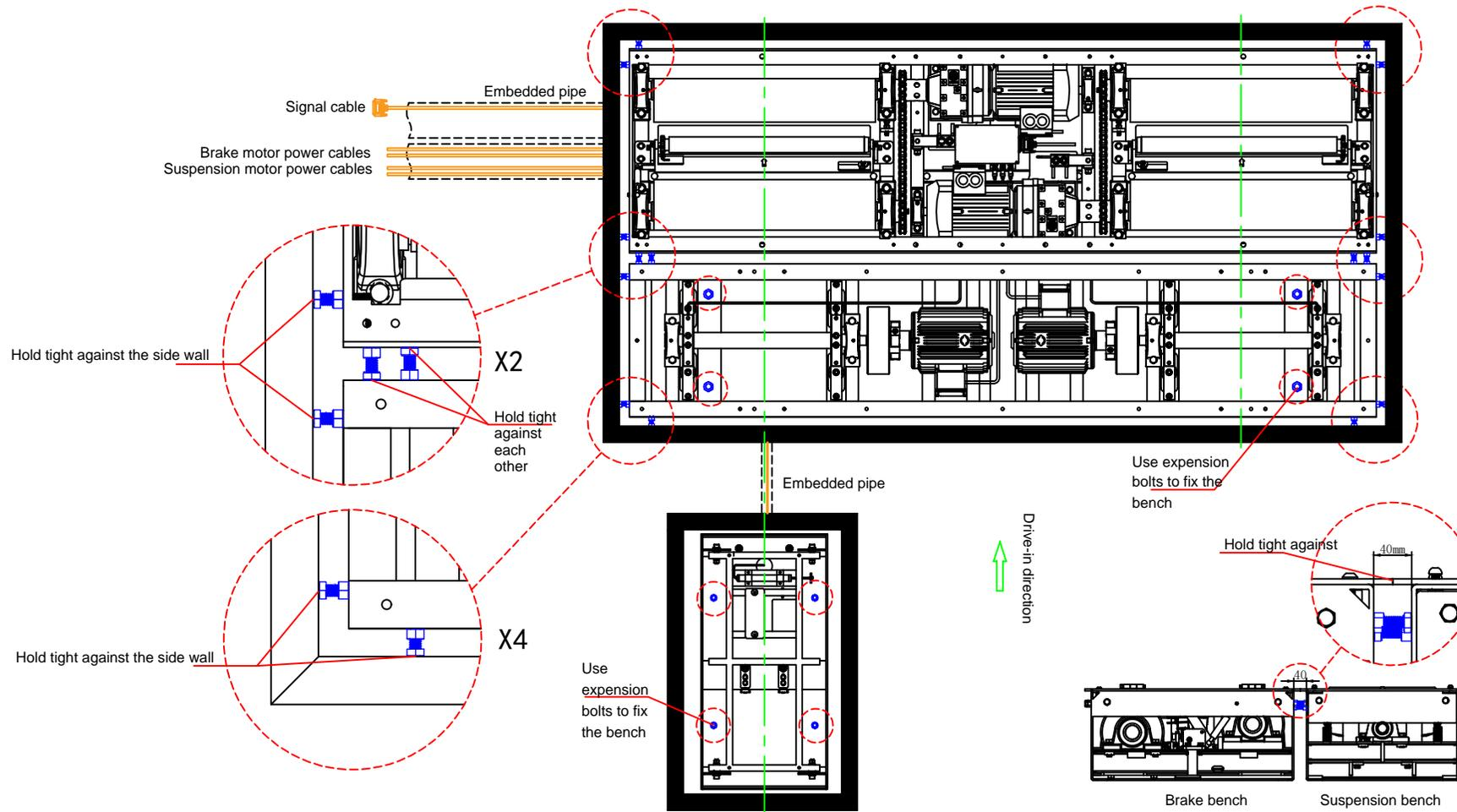
Adjust the position of the sideslip bench, make sure it's in the middle of the pit, the distance between the bench and pit should be same no matter in which side. Meanwhile, make sure that the direction of the bench is parallel with the drive-in direction. Then confirm the position of the expansion bolts, drill the holes, fix the bench ;
