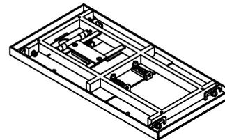
Remove the cover plate of the brake bench and suspension bench, and fit the eyebolt;
